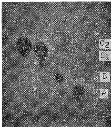
Fig. 1. Bioautograph of the megalomicin complex. Chromatogram run on thin-layer silica gel GF plates using the chloroform-methanol (3:2) system and plated against Staphylococcus aureus .
